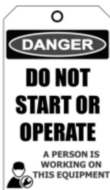
**DANGER TAGS** are used when someone is working on a piece of equipment. **DO NOT START** the equipment because someone could be hurt or killed.
